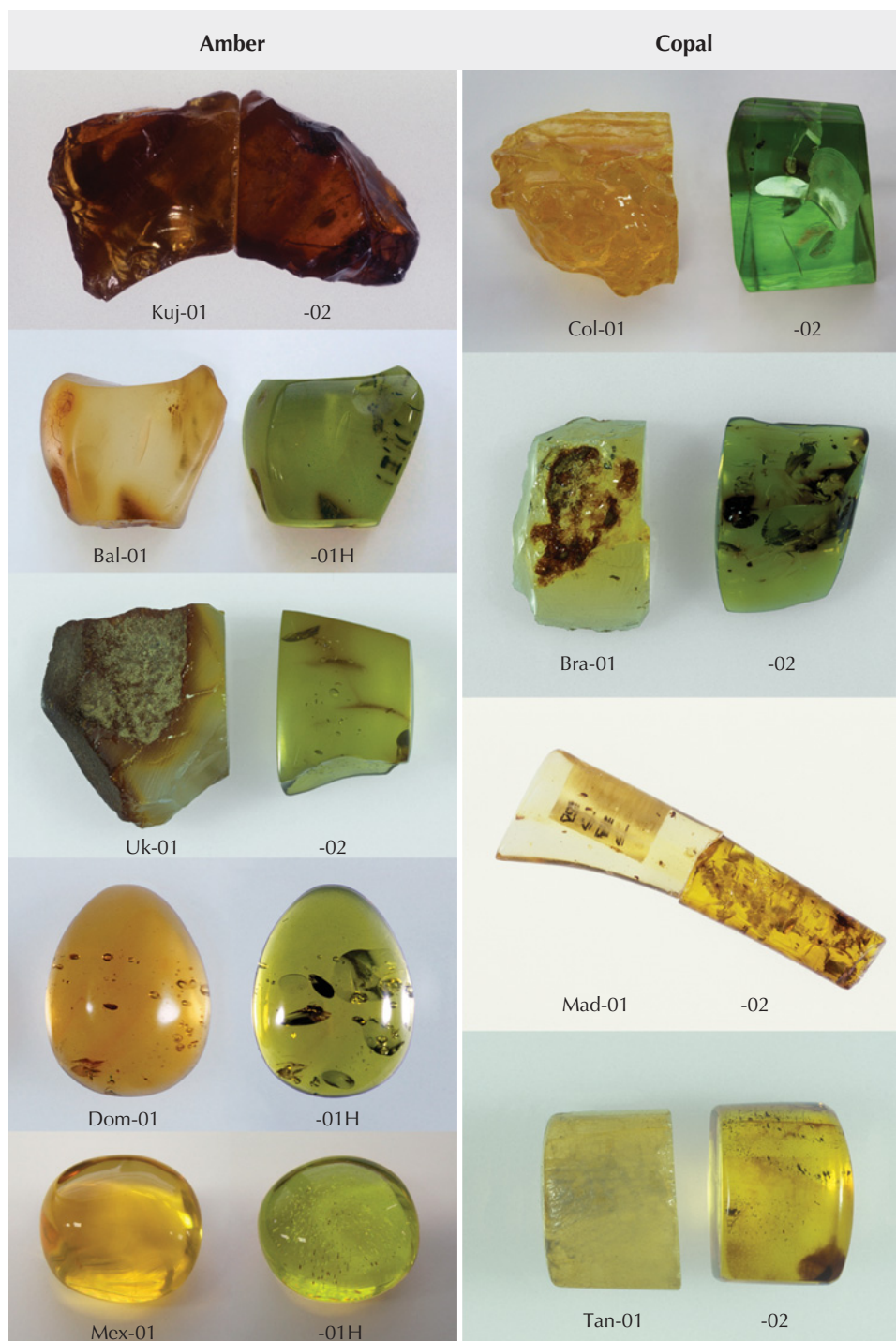
Figure 5. Representative amber and copal samples from various localities were used for the standard two-stage heating experiments. For each pair, the untreated samples are shown on the left, and those after heating are shown at the right. Colombian (Col-02) and Brazilian (Bra-02) copal turned bright green. Pale yellow copal from Madagascar (Mad-02) and Tanzania (Tan-02) turned intense yellow with a slight green hue. Kuji amber (Kuj-02) turned dark brown. Amber samples from the Baltic Sea region (Bal-01H) as well as from Ukraine (Uk-02), the Dominican Republic (Dom-01H), and Mexico (Mex-01H) generally turned green, although the color of the Dominican and Mexican material was not highly saturated. Photos by Masaaki Kobayashi.
